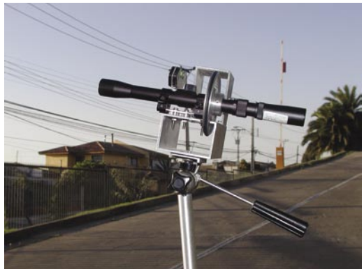
Angle finder to check luminaires installations
